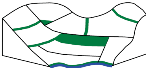
Figure 3. Examples of catchment restoration measures. Sediment traps (top left and right) are only effective if situated at the headwaters, near the source of eroded soils. Buffer zones for pesticide, P- and soil accumulation (bottom left) can effectively reduce the impairment of rivers from the catchments, if they are situated throughout the catchment. However, buffer strips alongside the main river alone have little effect. Constructed wetlands for denitrification, P-, and soil accumulation (bottom right) can be effective, if the conditions given in the picture are met. Cf. Syversen 2005; Gril & Lacas in: Braskerud 2005.
