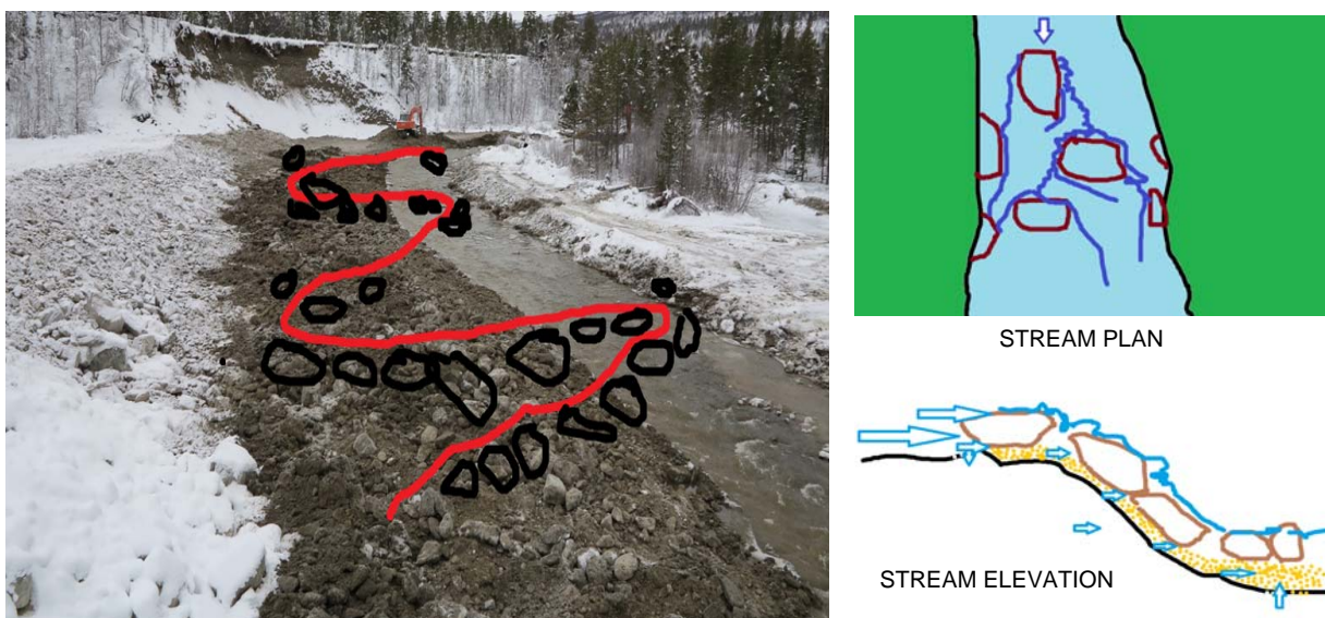
Figure 3. Making micro-niches and ensuring upward flow through sediments through introducing meanders and boulders.
