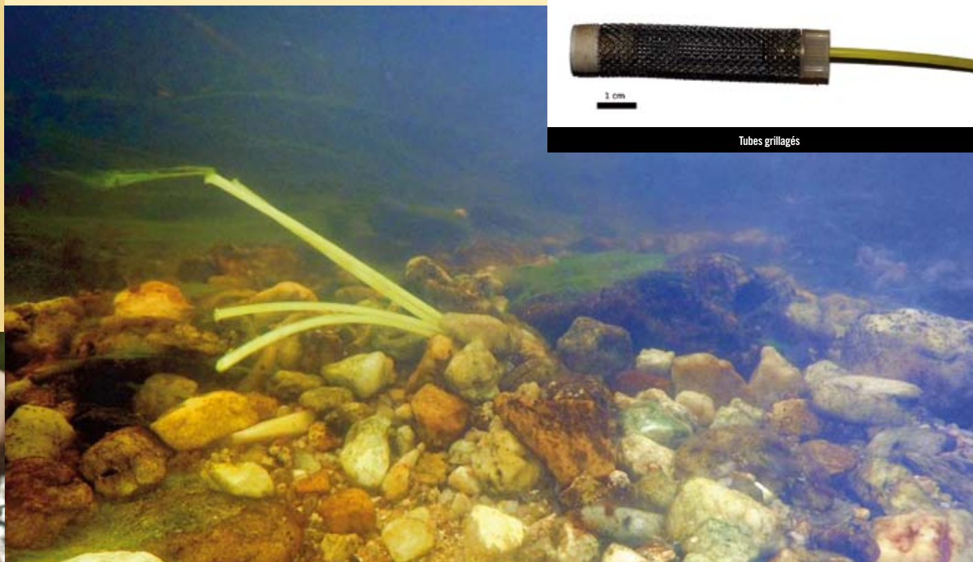
Tubes grillagés in-situ
